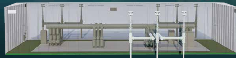
Conventional GIS prefabricated substation
