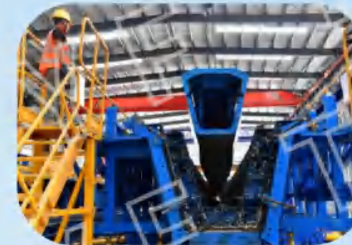
Box Girder Mold
