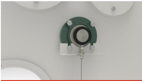
Cotton spinning machine speed detection
