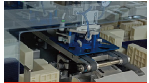
Vacuum chuck wafer presence detection
