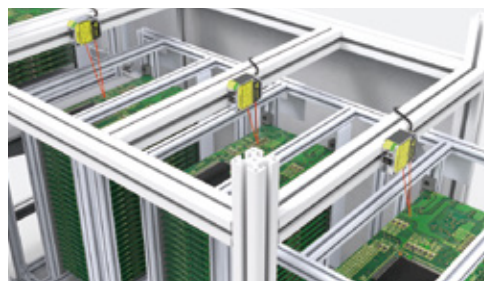
Sensing/Monitoring of PCB stacker height
