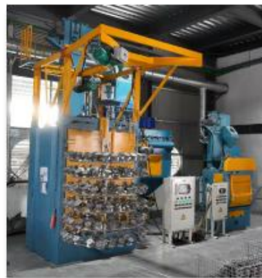
挂式抛丸机 Foundry-grade hook hanger design
