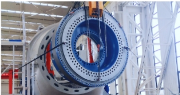
8MW直径3200mm风电设备三排柱主轴承吊装现场 Hoisting Site of 3200mm-Diameter Three-Row Cylindrical Main Bearing for 8MW Wind Power Equipment
