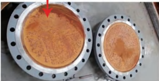
BEFORE BEING REMOVED
