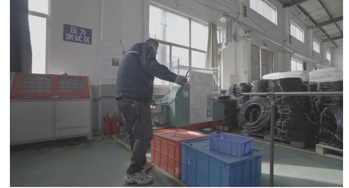
Water pressure test
