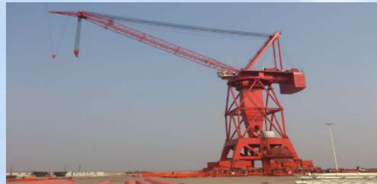
180t MQ Type Gantry Crane for Ship Building
