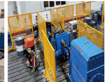
Transmission/torque converter /drive axle/wheel reduction assembly test bench
