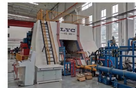
Shield Machine Main Bearing Test Bench Maximum Workpiece Size: \Phi 4800\text{mm}
