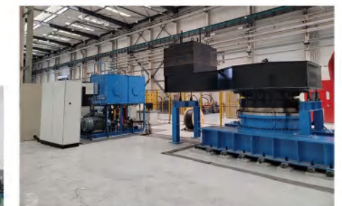
Construction Machinery Slewing Bearing Test Bench Maximum Workpiece Size: \Phi 1600\text{mm}
