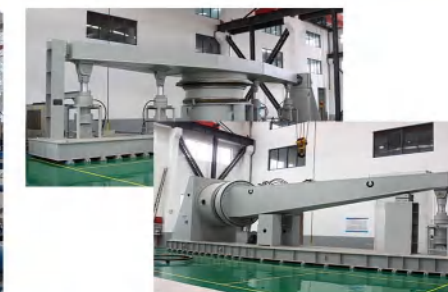
Wind Power Slewing Bearing Performance Test Bench Maximum Workpiece Size: \Phi 6500\text{mm}
