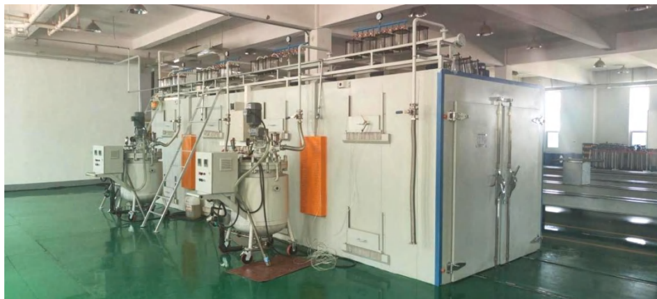
Vacuum Impregnated Insulated Busbar Production Equip.
