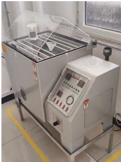
Salt-spray Test Equip.
