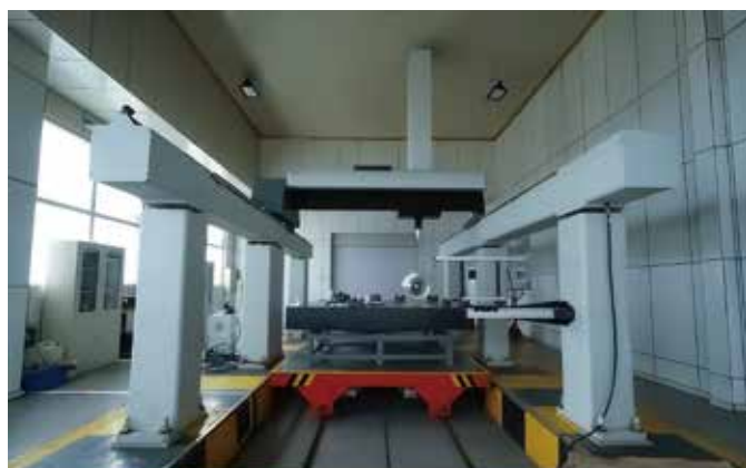
三坐标检测仪 5m*2.5m*2m CMM:5m*2.5m*2m
