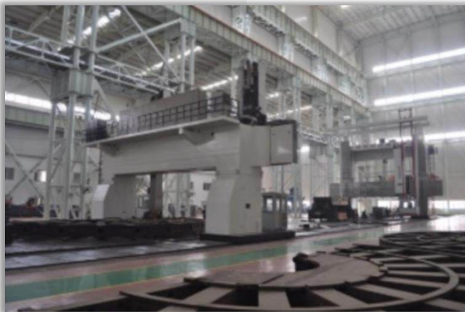
CNC double-gantry boring and milling
