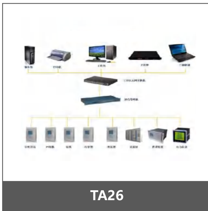
Substation Integrated Automation System
