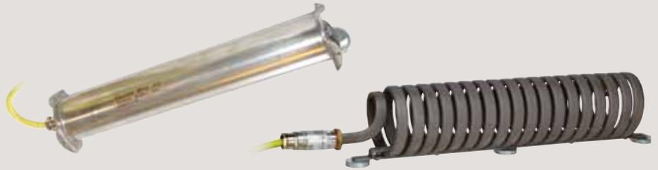
The NWC submersible oil heater is intended for preheating of hydraulic oil before start-up to minimize system wear. The preheating also reduces traces of water in the tank. Easy to use in existing oil tanks, there is no need for permanent installation. The oil heater is fastened at the bottom of e.g. the oil tank with integrated magnets.
