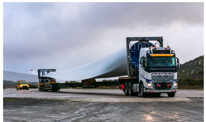
Fig. 2: The size of rotor blades and hubs are already causing high transport costs and expenses. (Image: AdobeStock_409306001)
