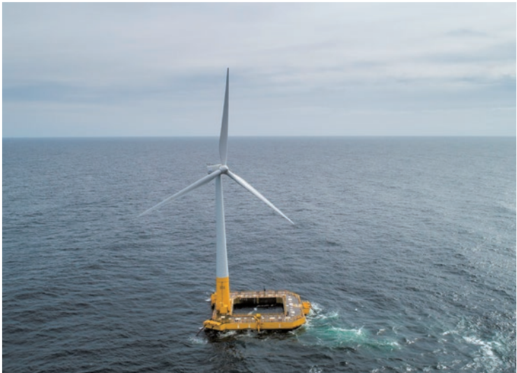
Image: Floatgen, Floating wind turbine equipped with the BW Ideol patented Damping Pool® foundation, operating in France for 5 years – Credits BW Ideol / V. Joncheray 注：本项目未使用本公司Floatgen的产品。
