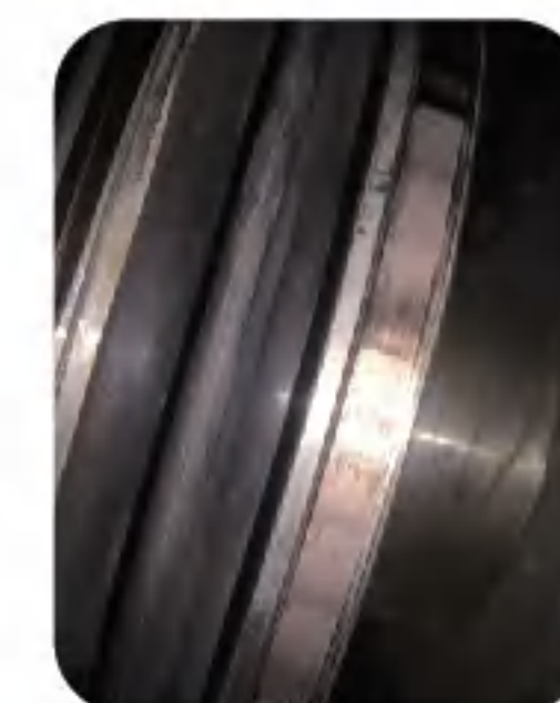
轴电蚀 Axial electro-corrosion
